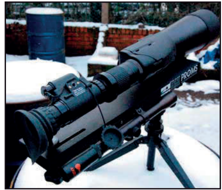
PROMS with optional PNP-M Night Scope Module for naked eye image intensified operation
