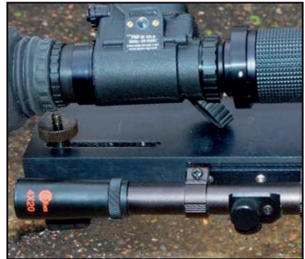
4 x 20 Finder Scope with cross hair mounted on rail (rail fitted to both sides of PROMS).
